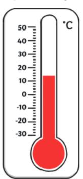
Most thermometers have small tubes and a bulb of liquid at the bottom. The hotter the temperature, the higher the liquid from the bulb rises in the tube. There are markings along the side of the glass tube that show the temperature.
